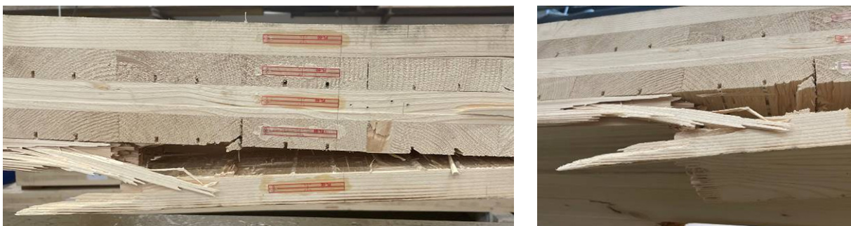
Fig. 8: Typical failure mode of Series A panels (specimen A2).
