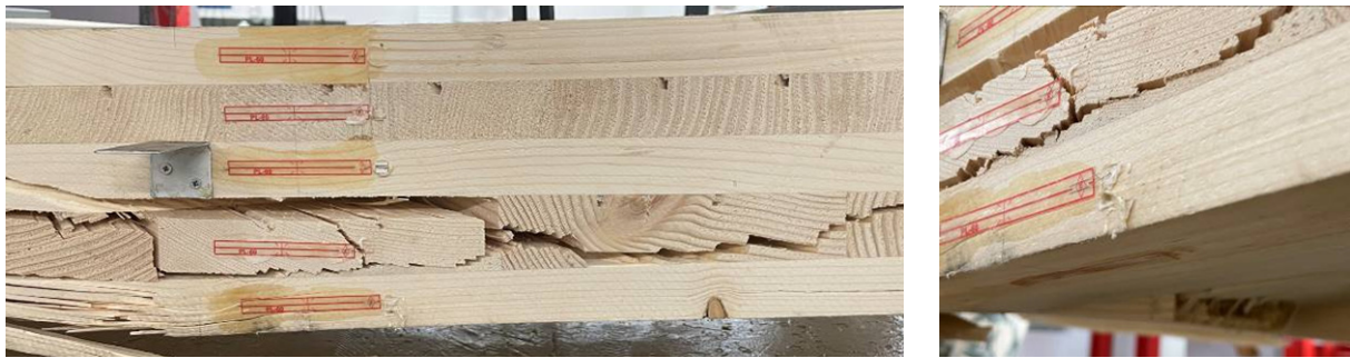
Fig. 9: Typical failure mode of Series B panels (specimen B1).
